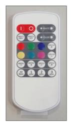
The battery disconnector must be removed before the remote control will operate. Only then can the wireless signal be sent.
