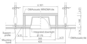
**Building material class:** A2-s1,d0 according to EN 13501-1 **Packaging unit:** 4 fire boxes per packet
