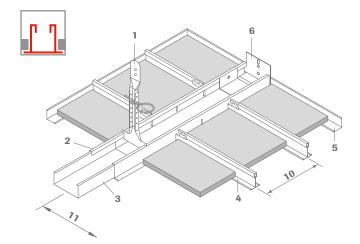
Nonius hanger no. 79/..., nonius hanger extension no. 16/... and safety pin no. 76
