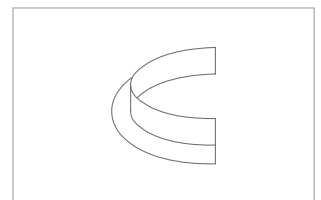
No. 8034/1 Pillar connection semi-circle \varnothing 250 – 500 mm in increments of 50; height: 20 mm, width: 20 mm, thickness: 1.5 mm Important: max. tolerance pillar diameter \pm 3 mm; adaptation required.
